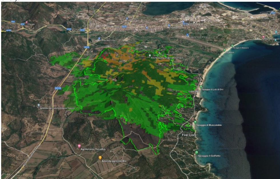
Figure 2: Map of the propagation speed of the Orri case study (July 13, 2019); the orange and red areas are characterized by propagation speeds exceeding 25 meters per minute.
