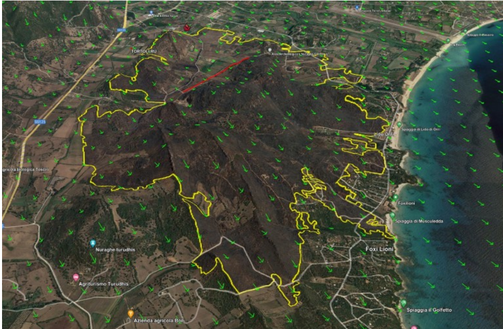
Figure 1: Wind field predicted by the meteorological model chain for the case study of Orri (13/07/2019).
